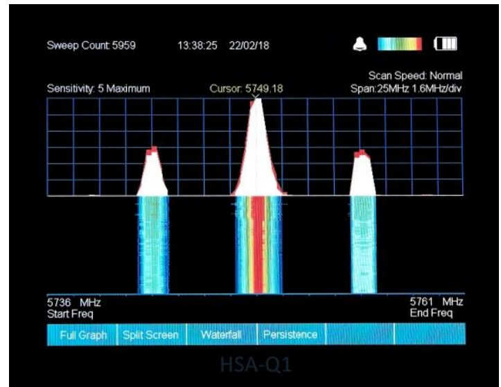
Split Screen (Half Waterfall) – Zoomed in to 25 MHz Span showing detected signal at 5.750 GHz
